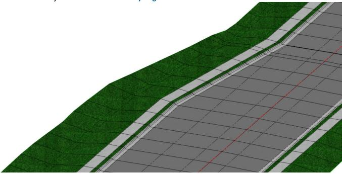
6. Rotate the 3D View to Top and note how the template drop changed direction and is now perpendicular the edge of pavement taper we defined as a Secondary Alignment.
