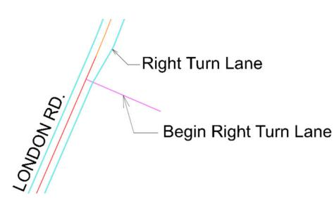
12. Review the 3D Model in the turn lane areas and note that the turn lane is not displayed. This is by design, in order for the turn lane to display you must add the edge of pavement as a corridor reference or create a point control to follow the edge of pavement.
