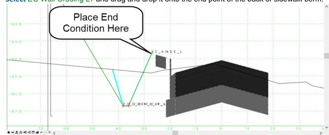
f. Select EC-Wall Grading LT and drag and drop it onto the end point of the back of sidewalk berm.
