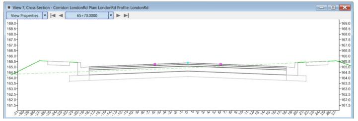
**Note:** This view window is showing dynamic cross sections extracted from the 3D model. All elements in the 3D model will appear in the cross section.
